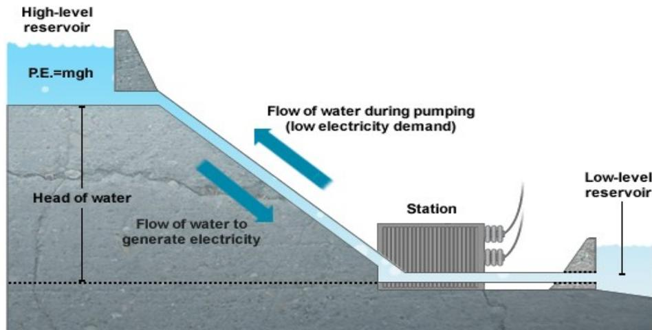
Fig. 9: Micro Hydro Power Unit Concept Diagram
