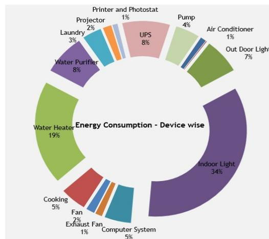
Fig. 13: Energy required for water pumping is at 4 per cent of total electricity use
