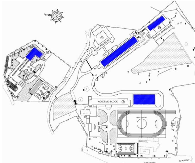
Fig. 6: First Phase SPV system of 50 kW (Blue strips in the middle)
